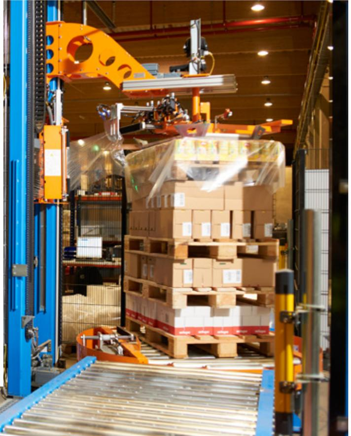
Well packed: The state-of-the-art logistics center has an automatic pallet stretch wrapper
